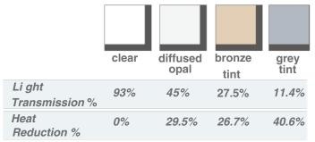
Light Transmission in accordance with AS/NZS 4257.4 standard test method. Heat Reduction in accordance with ISO 9050 Standard test method
